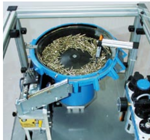
Fasteners are transferred from the bowl feeder to the placing head via the blow feeder
