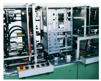
29 placing heads to assemble computer chassis using Speed Fastening® rivets.
