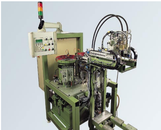
MIRS System to assemble vacuum pump
