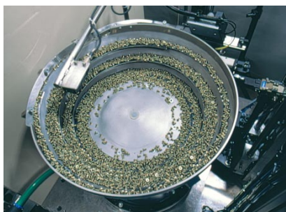
Fasteners fed via a vibrating bowl
