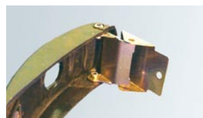
Composite material latch for wheel cover
