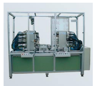
23 placing heads to assemble a computer chassis
