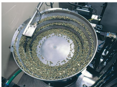
Fasteners fed via a vibrating bowl
